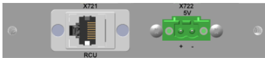
Figure 5: The RCU.I interface provides the 5 V supply as well as the direct link to the RCU.
