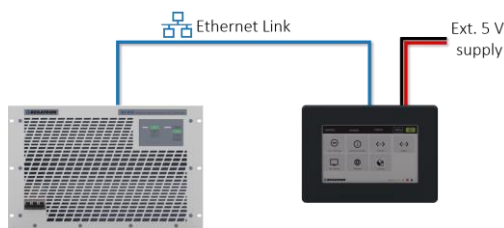
Figure 6: Direct link is possible to the LAN socket of the master device of a system. An external 5 V supply is required and the LAN socket is blocked by the link. External control is available via USB, analog interface or the optional CANmp interface.
