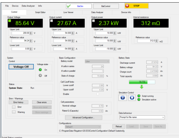
Figure 2: Information on the main operating values, like actual values and controller limits.
