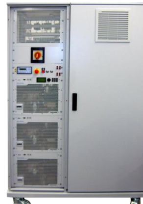
Modular Source/Sink power system 100 kW for utility vehicles year 2004
