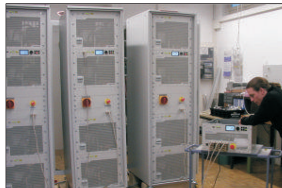
Multi Rack Controller MRC with 384 kW TopCon multi-unit system
