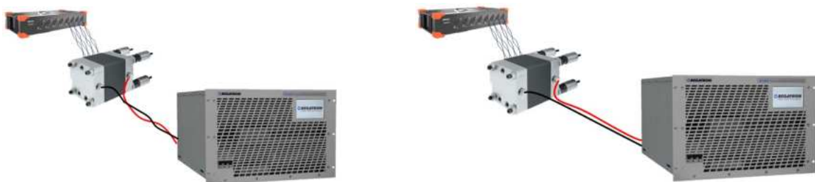
Figure 2: Wiring recommendations for correct measurements 2
